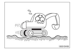
When working on soft ground, place mats or wood boards on the ground to prevent the machine sinking.
