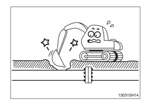
Check the locations of underground gas pipes or water line and secure the safety before operation. The operating near the electrical lines is very dangerous.
