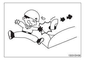
Do not open the engine hood and covers while the engine is running.
