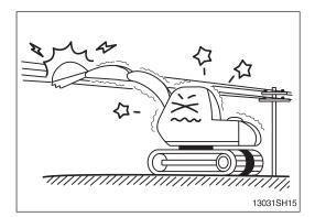
If the machine touches the electric power lines, keep sitting on the operator's seat and make sure the personnel on the ground not to touch the machine until turning off the electric current. Jump off the machine without contacting the machine when you need to get off.
