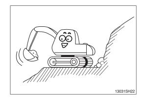
The swing on the slope can be danger of rolling over. Do not operate to swing the machine with the bucket loaded on a slope since the machine may lose its balance under such an instance.
