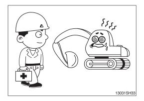
Park on a flat place and stop the engine for inspecting and repairing. Properly indicate that the machine is not operational (Remove the start key).
